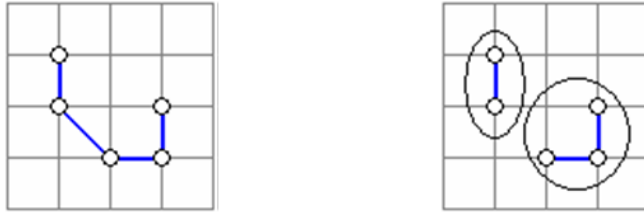
Fig.2. Minimal spanning tree and two clusters formed after elimination of the biggest edge.
